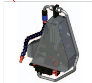
Roughing tool, activated by M codes. (SIGMA 32 only).
